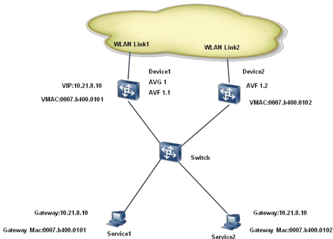
A GLBP group consists of Device 1 and Device 2, which bear the load balancing function of redundant gateways.
