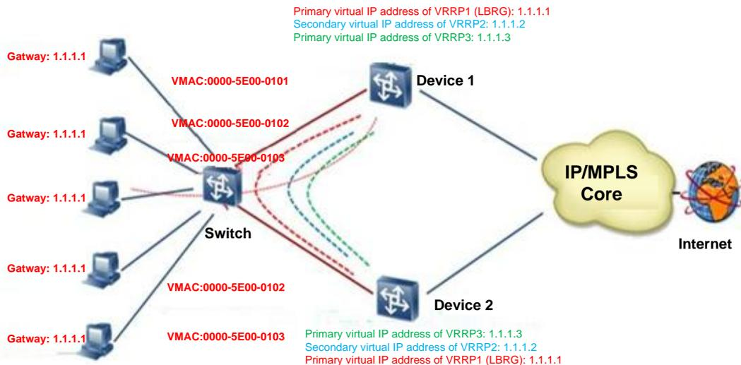
Implementation: LBRG uses a virtual IP address to respond to packets from different virtual MAC addresses. User traffic is directed to and load balanced among outbound interfaces based on virtual MAC addresses.
