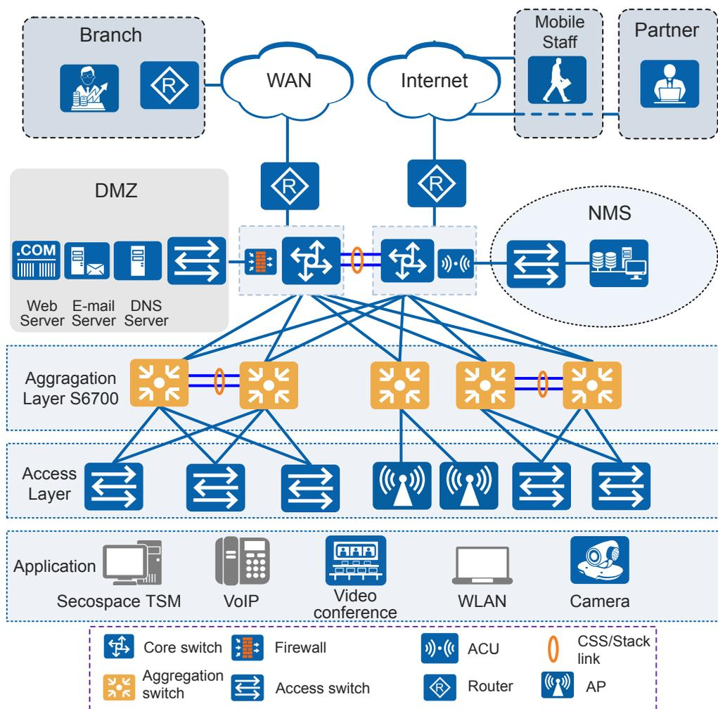
In an enterprise network or campus network, S6700 switches connect to access switches through 100M/1000M interfaces to provide high-performance switching and connect to core switches through 10GE optical interfaces. The network provides a 10G backbone layer and 100M-to-the-desktop capability, meeting requirements for high bandwidth and multi-service operation.
