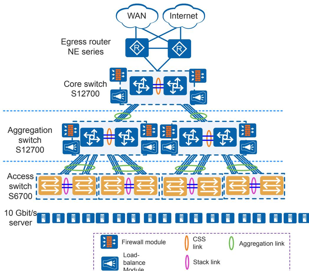
In a data center network shown in [Figure 2-1](#), NE routers act as the egress routers. S12700 switches work at the core and aggregation layers to ensure network security and implement load balancing using firewall and load balance modules.
