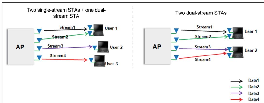
MU-MIMO is an outstanding feature of 802.11ac Wave 2, which depends on explicit transmit beamforming (TxBF). This feature requires that STAs support explicit TxBF. The reason is that when an AP concurrently transmits data to multiple users over the same frequency, signals are interference to users who are not target receivers of the signals. MU-MIMO uses TxBF to detect channels and uses precoding technology based on the feedback to mitigate such interference.
