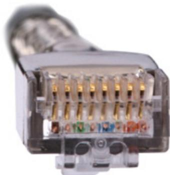
**Step 2** Hold an RJ45 connector at 45° to better visualize its metal contact strips. Ensure that the top edges of the metal contact strips are parallel. **Figure A-65** shows an unqualified connector with uneven metal contact strips.
