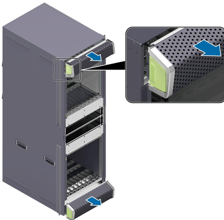
**Step 4** Remove the air filter from the SFU area.
