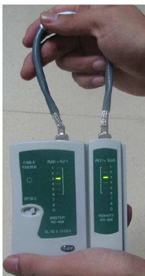
The procedure for testing a crossover cable is the same as that for testing a straight-through cable except for the sequence in which the indicators turn on. For that sequence, refer to crossover cable wire connections.
