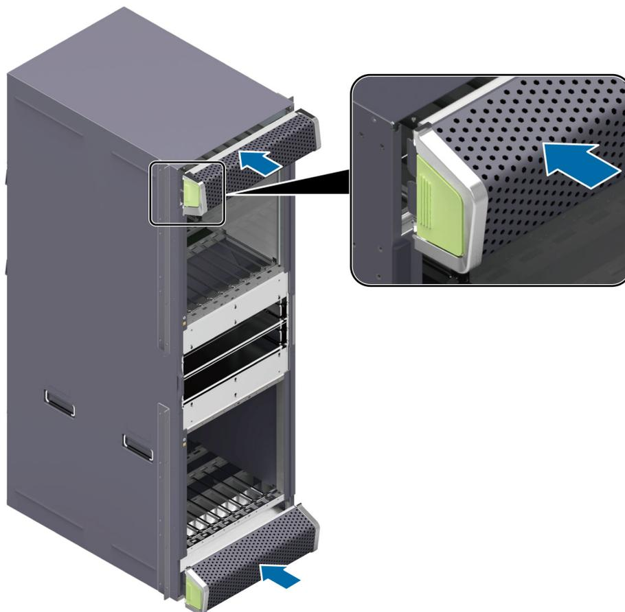
**Step 6** Install an air filter in the SFU area.
