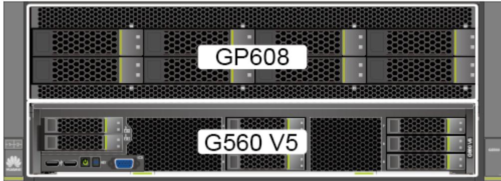
**Figure 1-5** Installation positions of the G560 V5 and GS608
