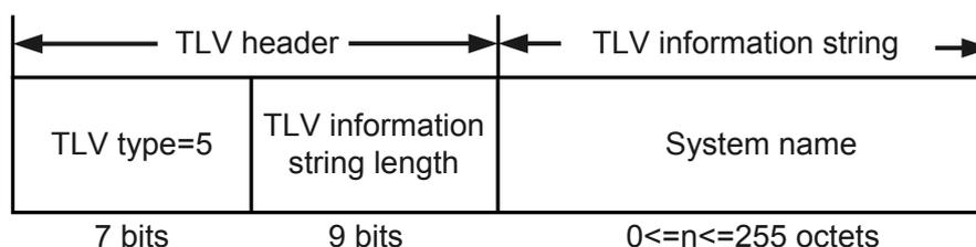
A System Name TLV contains TLV type, TLV length, and TLV information string, without a subtype. A System Name TLV identifies the complete domain name of the local device. If the LLDP agent complies with IETF RFC 3418, the System Name TLV value is the same as the sysName value in IETF RFC 3418. An LLDPDU contains only one System Name TLV.
