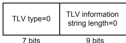
When the port status changes, for example, LLDP is disabled or the port is shut down, the port sends an LLDPDU with the TTL value of the Time to Live TLV set to 0 to the neighboring nodes. This LLDPDU is a shutdown packet. An End of LLDPDU TLV has only the type and length fields and does not have the field TLV information string. The type value of End of LLDPDU TLV is 0 and occupies 7 bits. The length of End of LLDPDU TLV is 0 and occupies 9 bits.
