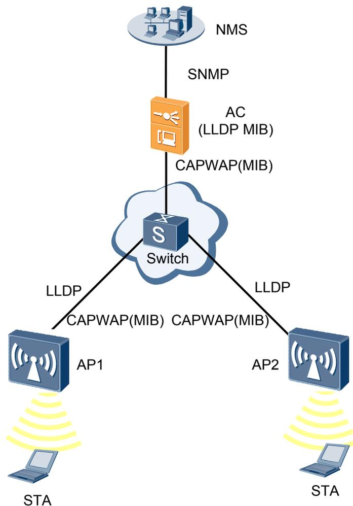
LLDP is enabled on AP1 and the switch. The process of LLDP topology discovery between directly connected neighbors is as follows:
