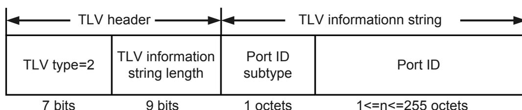
The type value of Port ID TLV is 2 and occupies 7 bits. The field TLV information string length indicates the TLV length and occupies 9 bits. The first byte of the TLV information string indicates the TLV subtype, and the others indicate the TLV content of 1 to 255 bytes.
