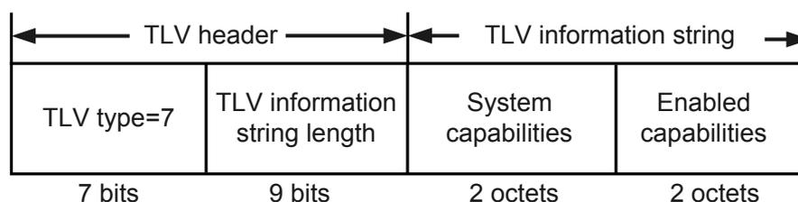
A System Capability TLV describes the functions that the system supports and has enabled. The TLV header of a System Capability TLV is similar to those of other TLVs. The resting fields of the System Capability TLV map different functions. **Table 2-4** describes the bits identifying the functions.
