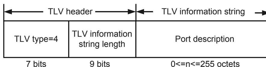
A Port Description TLV contains TLV type, TLV length, and TLV information string, without a subtype. The Port Description TLV identifies the description of a port on the local device. If the LLDP agent complies with IETF RFC 2863, the Port Description TLV value is the same as the ifDesc in IETF RFC 2863. An LLDPDU contains only one Port Description TLV.
