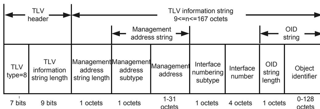
A Management Address TLV is used to advertise the management address of the local device. The value of TLV information string indicates the available type and value of the management address.
