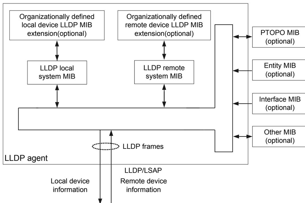
Four MIBs are used for information exchange with the LLDP module, including PTOPO MIB, Entity MIB, Interface MIB, and Other MIB. The LLDP module exchanges information with these MIBs to update its LLDP local system MIB and define the organizationally defined local device LLDP MIB extension. The LLDP module then sends LLDPDUs to the peer device to notify it of the local device information.
