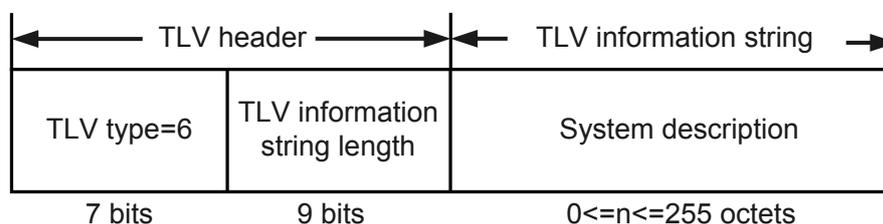
A System Description TLV contains the fields TLV type, TLV length, and TLV information string, without a subtype. The System Description TLV identifies the full name, system hardware version, operating system, and network software of the local device. If the LLDP agent complies with IETF RFC 3418, the System Description TLV value is the same as the sysDesc value in IETF RFC 3418. An LLDPDU contains only one System Description TLV.
