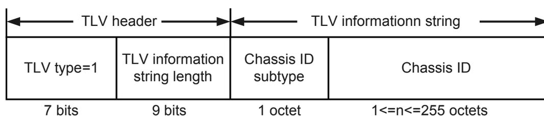
The type value of a Chassis ID TLV is 1 and occupies 7 bits. The field TLV information string length indicates the TLV length and occupies 9 bits. The first byte of the TLV information string indicates the TLV subtype, and the others indicate the TLV content.
