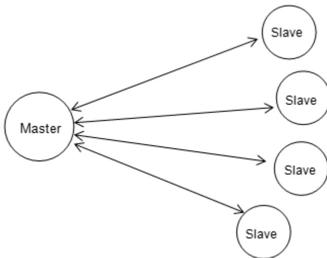
The master and slave devices communicate with each other in wireless mode. On an IoT AP, the master device uses the AP's uplink network interface to communicate with the Bluetooth server. BLE works in the 2.4 GHz frequency band and occupies 40 channels with 2 MHz bandwidth per channel. Three are fixed advertising channels, and 37 are data channels that support Frequency Hopping (FH).
