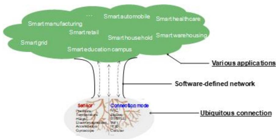
In an IoT network, various types of sensors collect information from the physical world (information obtaining), and send the information to various types of intelligent applications (information transfer). These intelligent applications then process the information and perform decision-making (information processing). Next, they share the decision-making results with the physical world to ensure that the focused objects work as expected (generation of information effects).
