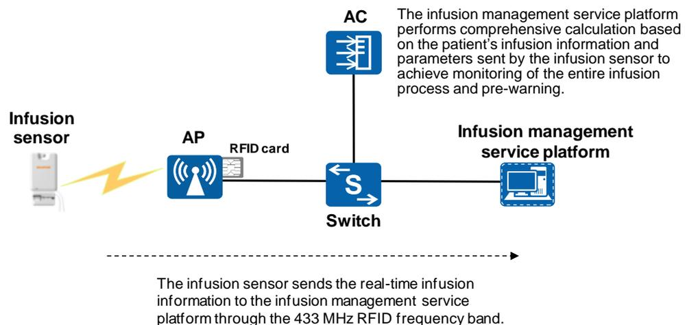
When a patient receives infusion treatment in a hospital, the patient wears a wristband. The patient's basic information, diagnosis information, bed number, infusion treatment information, and infusion process are recorded into the database. A handheld terminal is used to scan the barcode on the patient's wristband to obtain the patient's infusion treatment information from the database.
