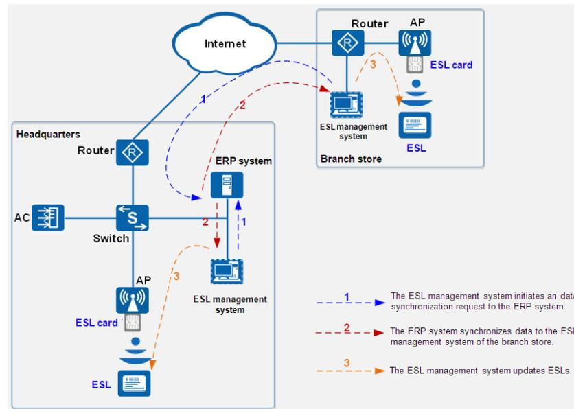
The ESL management system needs to interwork with the customer's Enterprise Resource Planning (ERP) system so that information such as product codes and prices can be synchronized to the ESL management system. The ESL operation process follows:
