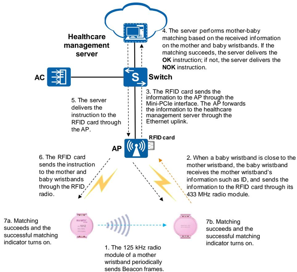
1. Mother wristbands and baby wristbands are bound and paired on the backend server. The 125 kHz radio module of a mother wristband periodically sends Beacon frames.
