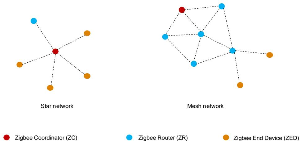
Nodes in Zigbee topologies are classified into Zigbee Coordinator (ZC), Zigbee Router (ZR), and Zigbee End Device (ZED). ZC is responsible for building and managing the entire network. After the network is built, ZC is also a ZR, which provides routing information and can allow other devices to access the network. ZED is an end node and is not responsible for network maintenance.
