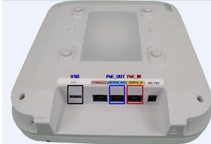
**Figure 2-3** Physical interface 2 of an IoT AP
