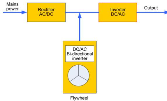
**b). Rotary online fly wheel UPS (typical example: Piller solution)**
