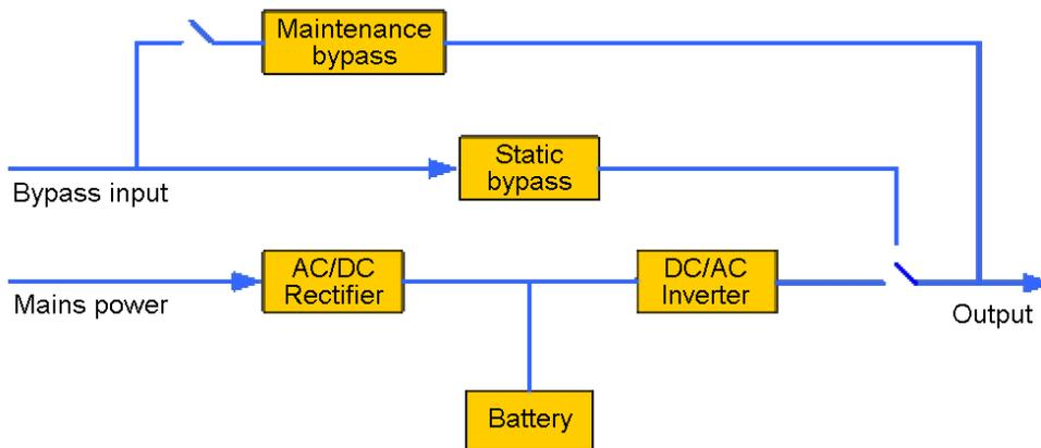
An UPS has multiple working states including the normal mode, static bypass mode, battery mode, and maintenance bypass. The online double conversion UPS can be classified into the transformer-less UPS and transformer-based UPS by structure, which will be described in this document.
